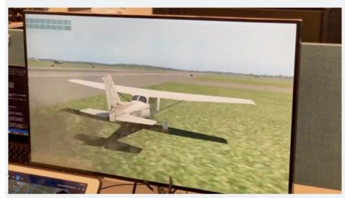
Enlarge / A plane in the researchers' demonstration attack as spoofed ILS signals induce a pilot to land to the right of the runway.
